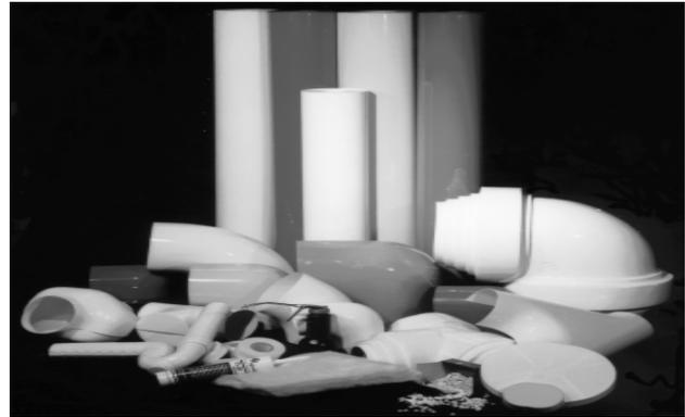
Speedline® Smoke Safe™ PVC Insulated Fitting Covers and Jacketing are designed for applications indoors or out-of-doors in commercial, institutional and industrial facilities. The system has an applicable temperature range of -35°F to 500°F (-37°C to 260°C). The PVC surface should remain below 150°F (66°C) through the installation of sufficient insulation on higher temperature applications.
